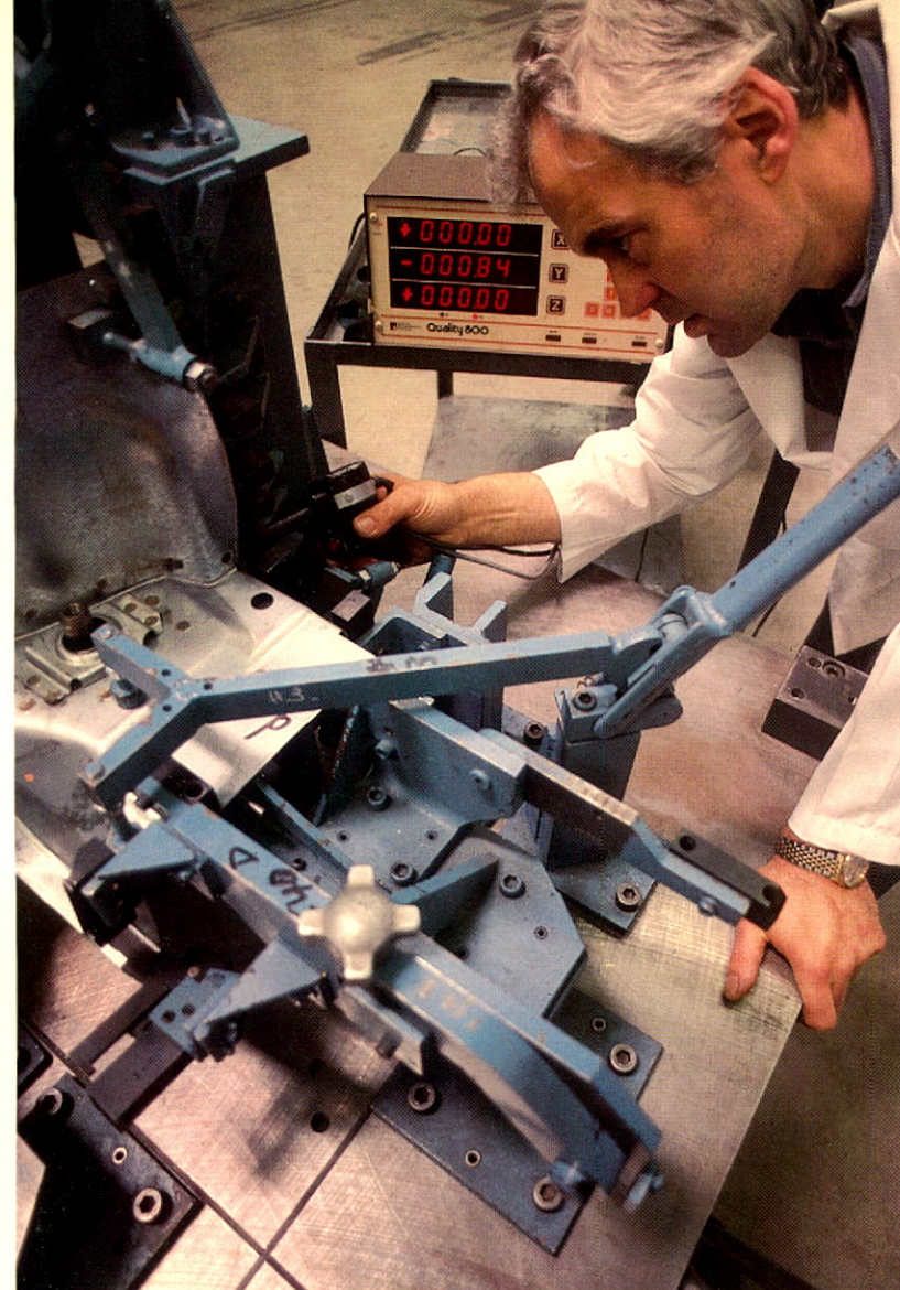
Opposite page: Employees actively participate in the SPC process during production. Left: Statistical process control (SPC) fixture for large chassis stamping panel. Right: Co-ordinate measurement of rear crossmember assembly. Lower: Robotic welding lines are designed and built by our new MTE Group.
