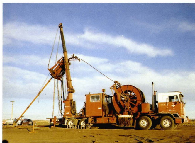
Logging in deviated well with coiled tubing.
