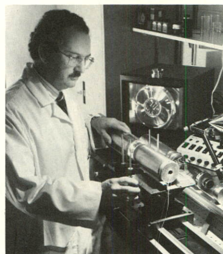
ALAIN SPÉNARD CHECKS THE TELEGEOMETER USED TO INSPECT BOREHOLES (ELECTRONICS, IREQ).
