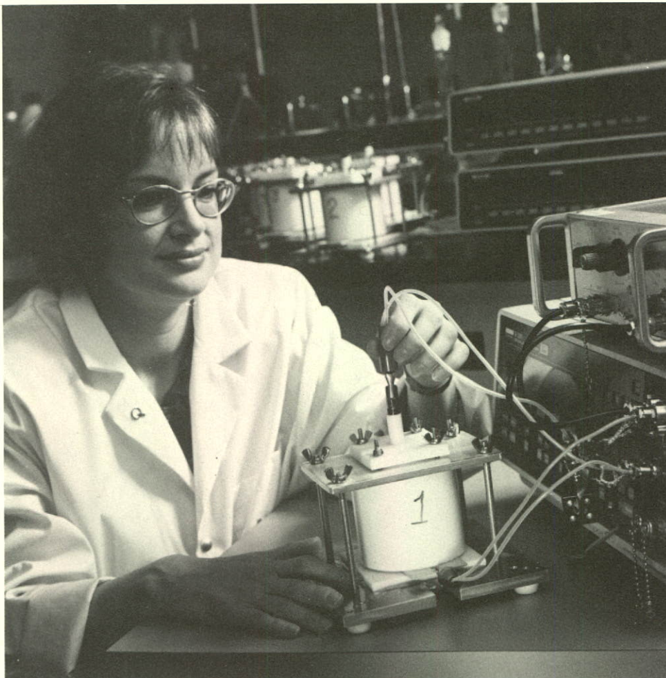
ESTELLE POTVIN USES ELECTROCHEMICAL IMPEDANCE SPECTROSCOPY TO TEST THE PAINT ON A STEEL SPECIMEN (MATERIALS CHEMISTRY, IREQ).
