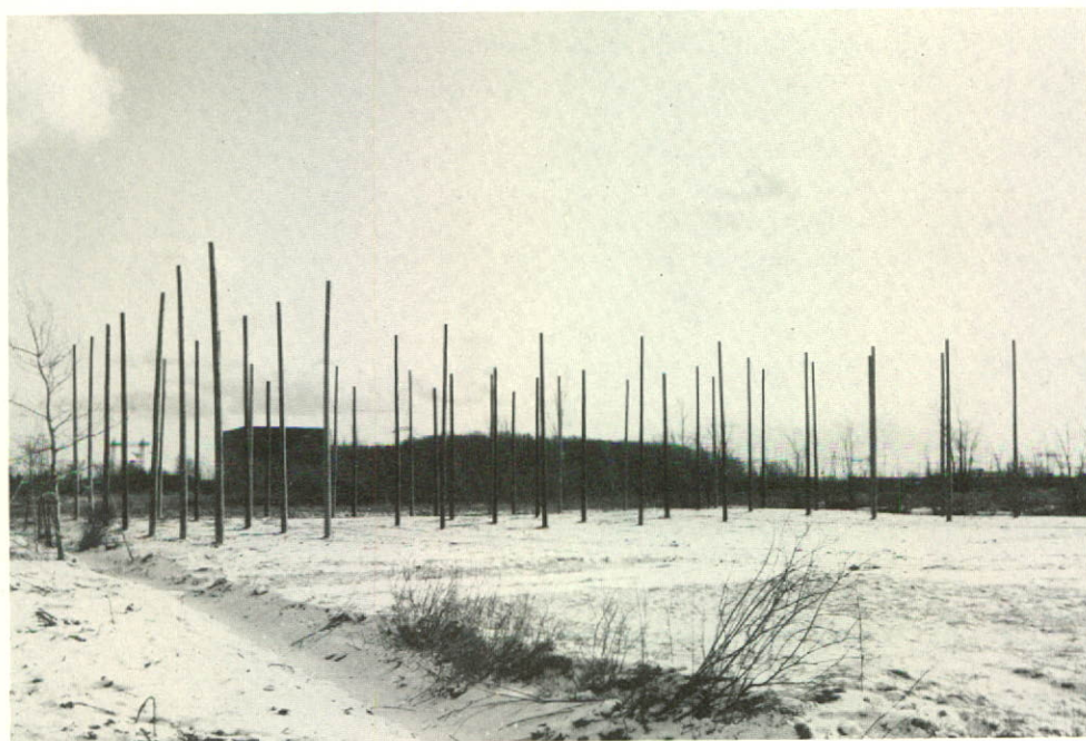
WOOD POLE TESTING TAKES PLACE UNDER REAL CLIMATIC CONDITIONS (MATERIALS CHEMISTRY, IREQ).
