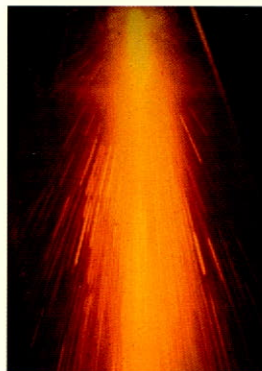
Gas Atomization Producing Powdered Metals
