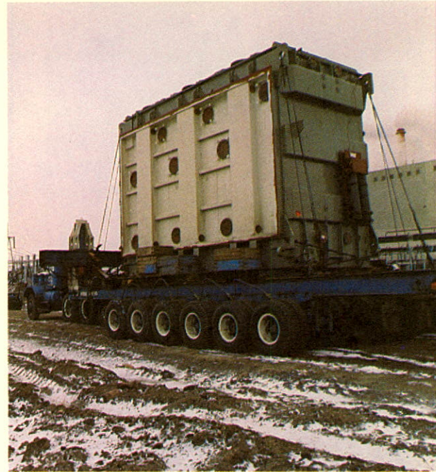
A tie-line for seasonal exchange of power with North Dakota requires use of advanced facilities including this massive phase-shifting transformer near Estevan.
