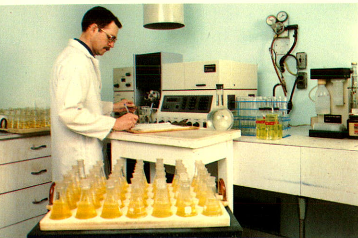
Atomic Absorption assay analysis used to determine base metal grades and lower grade gold values.
