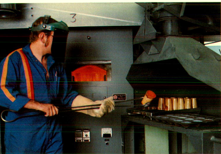
Fire Assaying of gold orebody drillcore to determine the gold grade.
