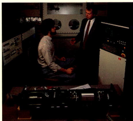
A controlled atmosphere welding system is undergoing assembly. The system incorporates a JK Laser solid-state Nd:YAG laser (foreground) for producing high quality welds in a nitrogen filled chamber (center at back of photo).
