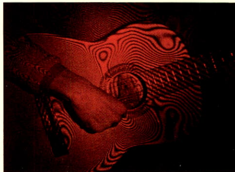
Dark interference fringes on this double pulse hologram show vibrational movement of the guitar soundboard. Holographic interferometry can be used in a similar way to analyze vibration in engineering structures.
