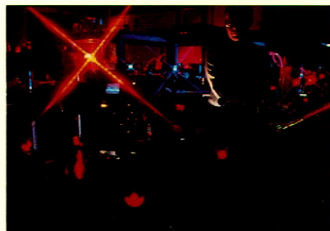
A Lumonics Excimer laser in use by Doctor Paul Corkum at the National Research Council, Ottawa, as an amplifier for ultra-short picosecond pulses.
