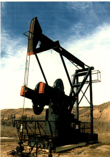
Pumpjack at the West Eagle Unit in British Columbia.
