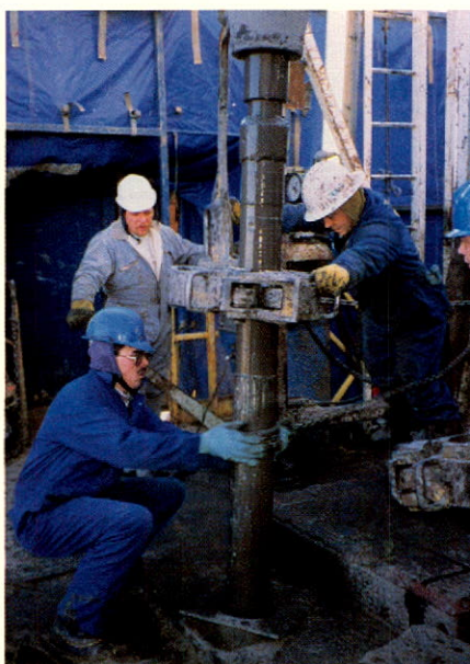
Rig crew connects drill pipe at Ring/Border, northeastern British Columbia.
