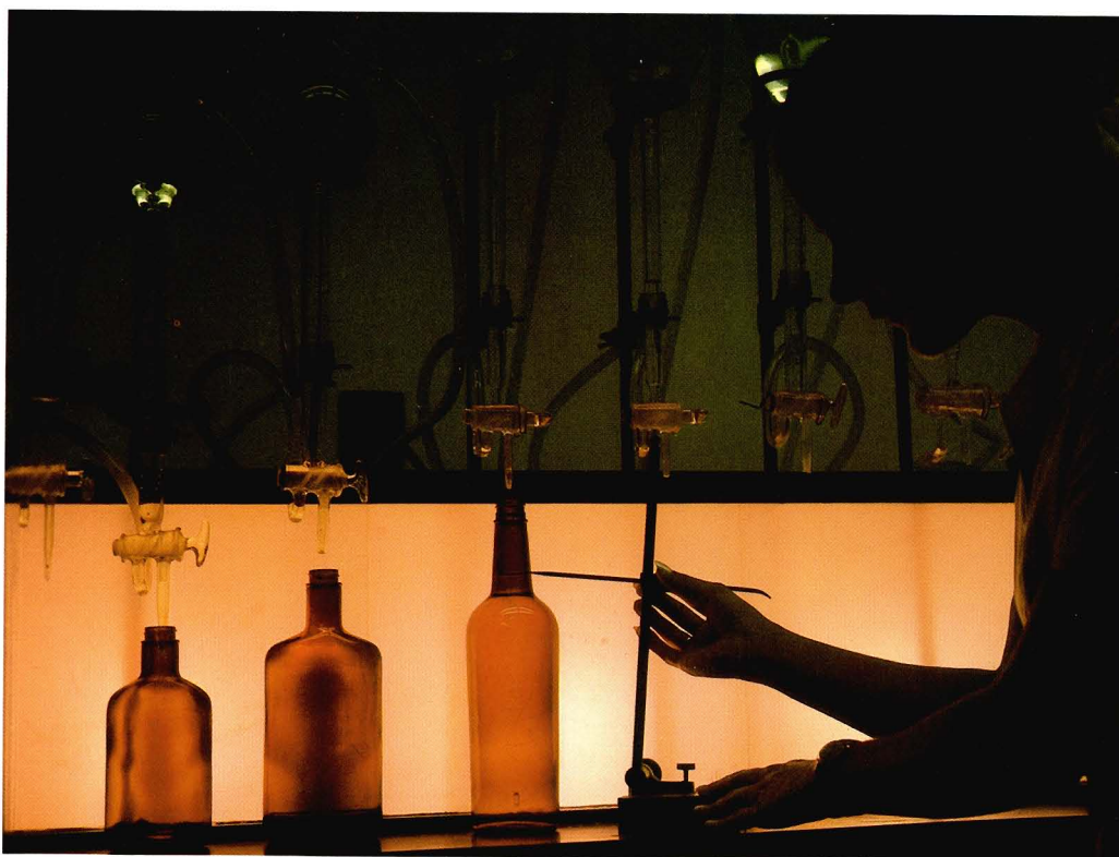
Any imperfect bottles are detected here.
