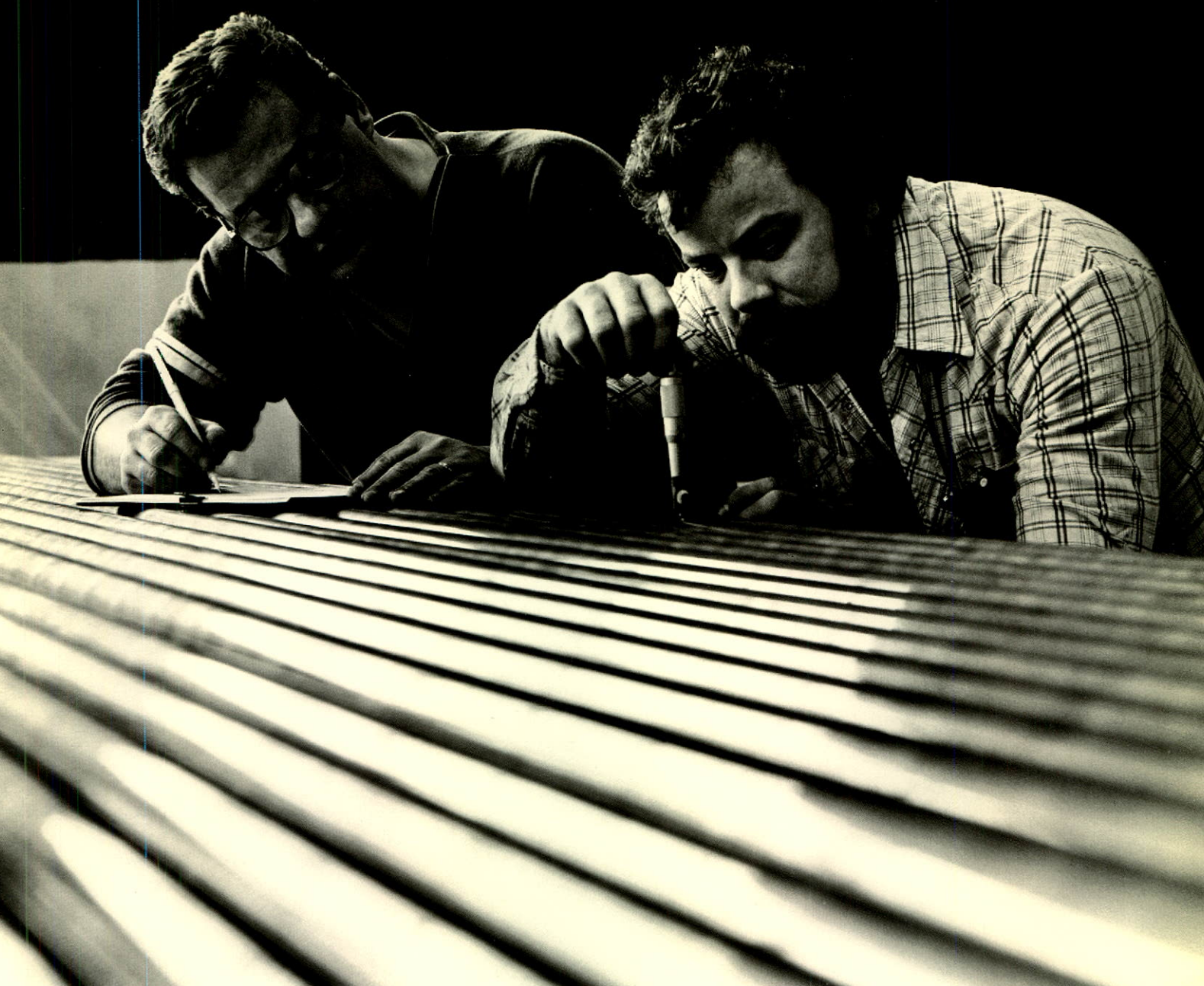
Cupronickel tubing, used in shipbuilding for the U.S. Marines, gets final quality inspection at N.M.I.'s Montréal East plant by André Sarrazin Jr. and Robert Bettner.
