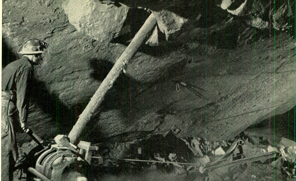
Tugger hoist scraping ore to a drawpoint.
