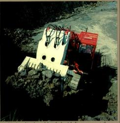
Hydraulic shovel loaded with limestone at the Paulding Cement Plant.
