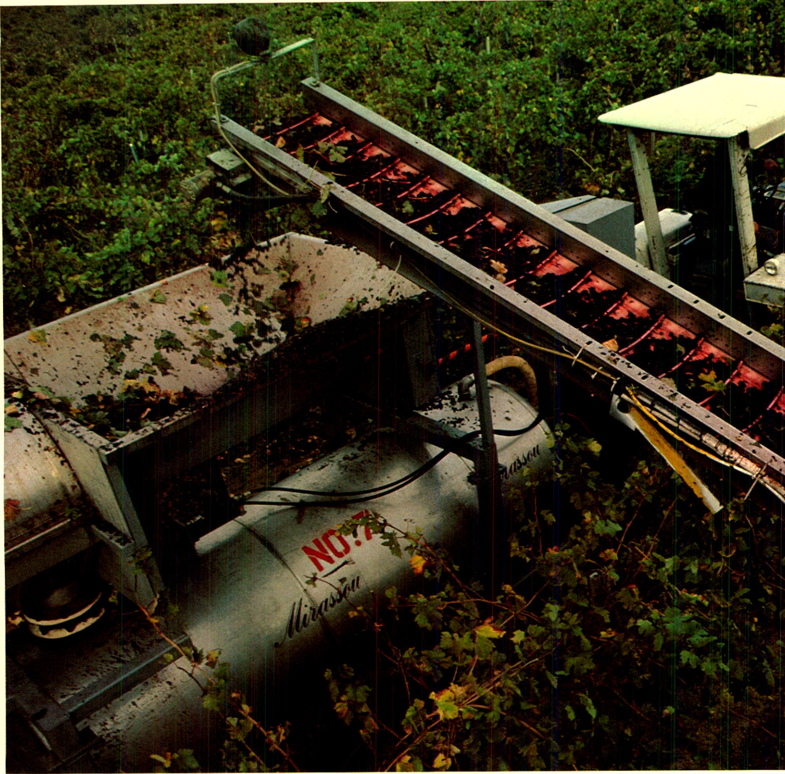
Above: Automatic grape harvester sends grapes along conveyor to 1,000-gallon tank made of 10-gauge Crucible stainless steel. Tanks are made by Valley Foundry for Mirassou vineyards, Monterey County, California.
