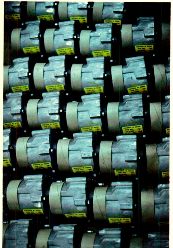
Below: Emissions control pumps for the automotive aftermarket ready for shipment from Holley Special Products Division. Pumps inject air into car exhaust systems to help reduce pollutants.
