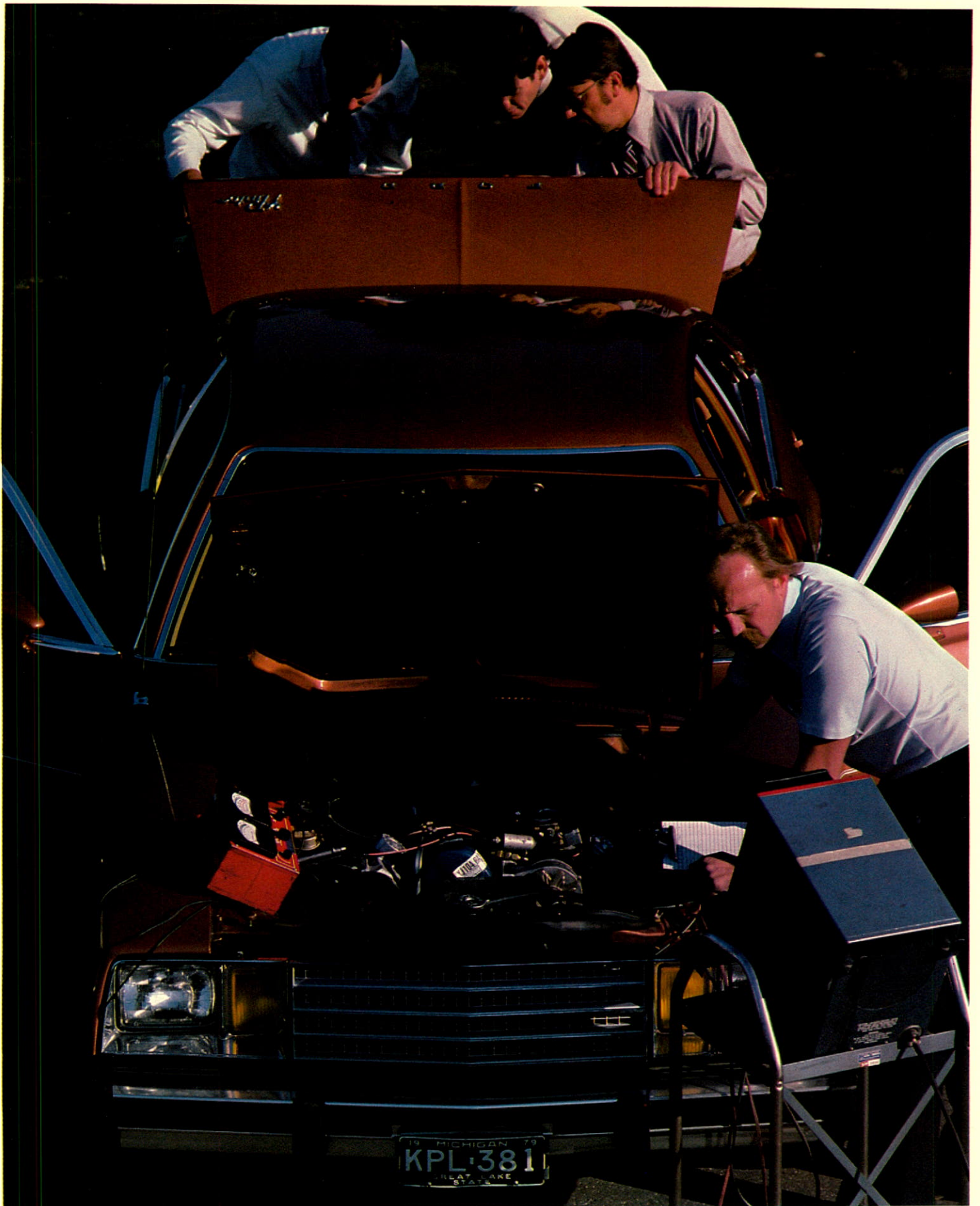
Holley test car, equipped with Holley single-point fuel injection system, is examined by engineers. System delivers incoming air at sonic speed and uses no moving parts other than conventional throttle plates.
