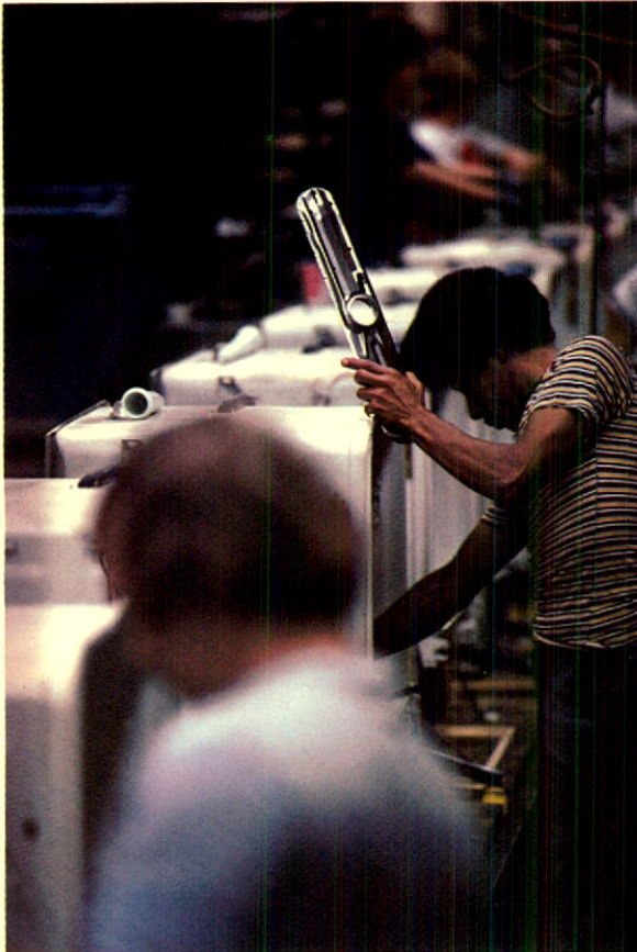
Above: Crucible stainless steel is used to manufacture rotating spray arms for General Electric automatic dishwashers, shown here during assembly at Appliance Park near Louisville, Kentucky.
