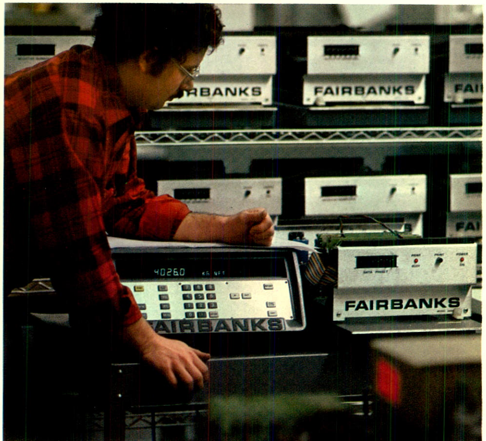
Below: New Fairbanks weighing products, the Datacenter 8811 and Datapage 3600 printer, are elements of micro-processor-based system that provides digital display, memory, and data accumulation.
