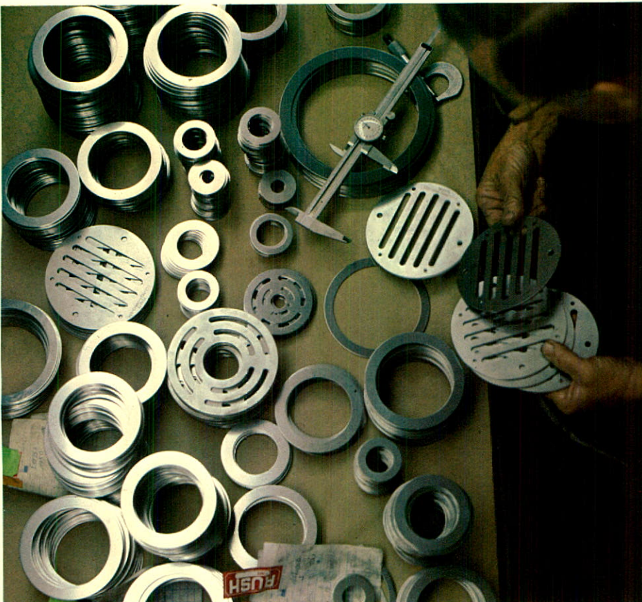
Above: Each compressor valve, ring, and seal made by France Compressor Products Division is inspected for dimension, finish, and sealing surface. Products are sold as original equipment and as replacement parts for air and gas compressors.
