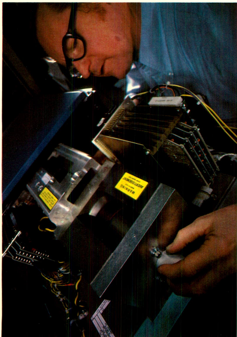
Left: Technician adjusts fractional horsepower linear motor that relies on Crucible alnico magnets. Motor actuates the read-write head in a Control Data Corporation storage module disc drive.
