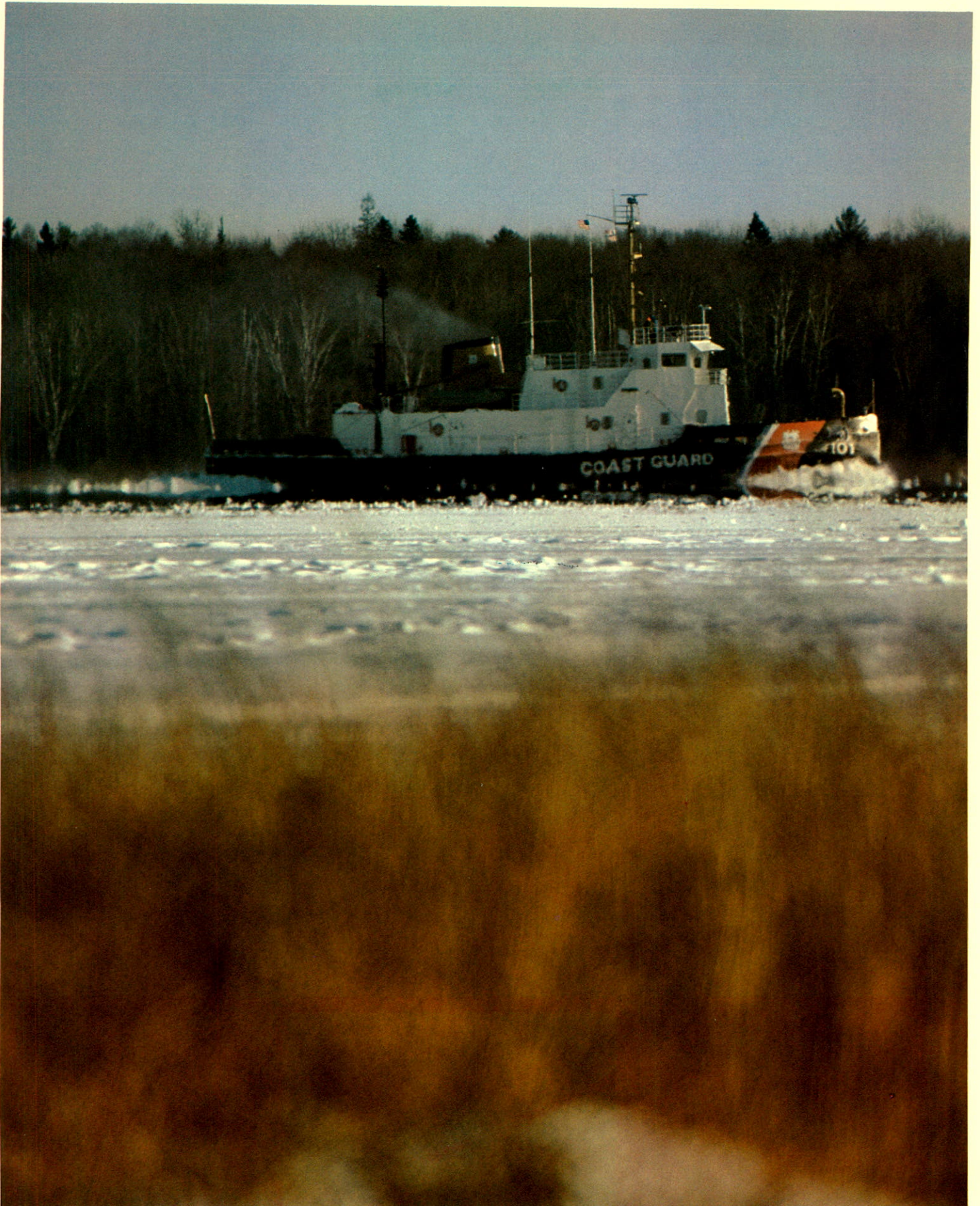
U.S. Coast Guard cutter Katmai Bay , one of a new class of ice-breaking tug designed to help keep Great Lakes shipping channels open in winter, is powered by two Fairbanks Morse opposed piston diesel engines.
