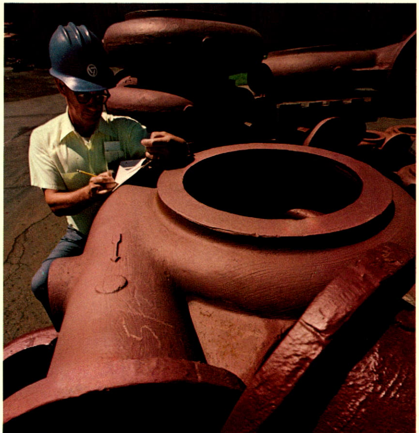
Below: Fairbanks Morse non-clog vertical and horizontal angle-flow pump casings are inspected. The division produces pumps for industrial, public works, agricultural, and domestic use.
