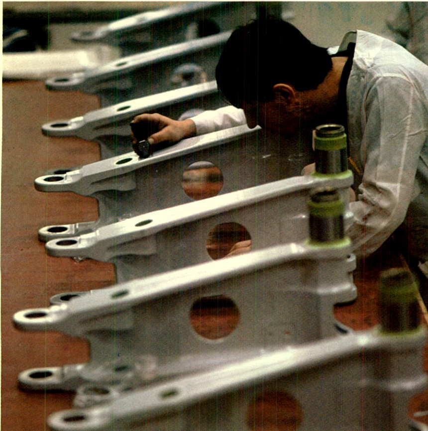
Above: Main landing gear side-support struts for Boeing 727 jetliners are stamped with production numbers at Menasco Canada Ltée in Montreal. Menasco Canada landing gear is also widely used on commuter aircraft.
