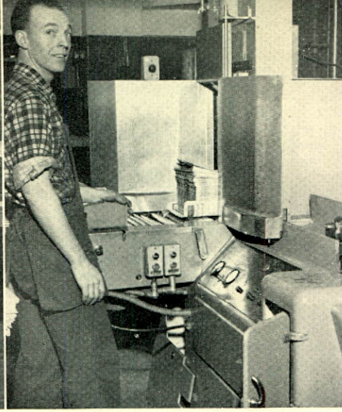
This machine ties bundles with one strand of wire, electrically welded into a neat join.
