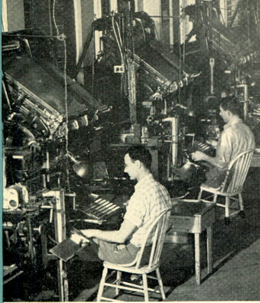
Batteries of linotype machines are essential equipment in the production of a newspaper.
