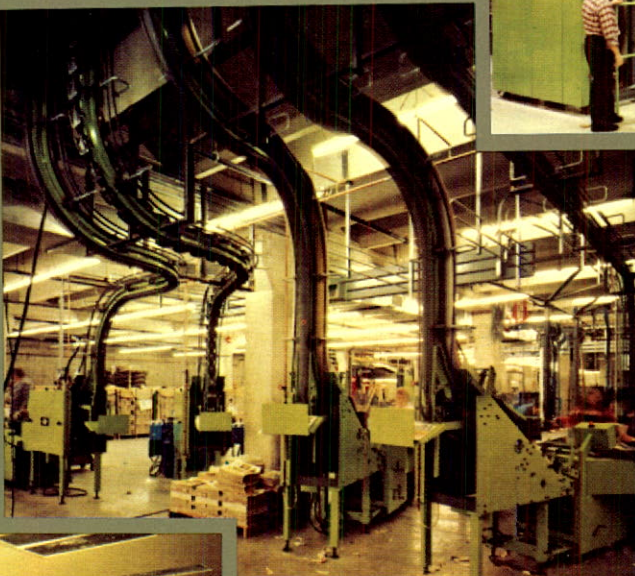
The complex conveyer system at The Herald delivers newspapers from the presses to the mailroom.
