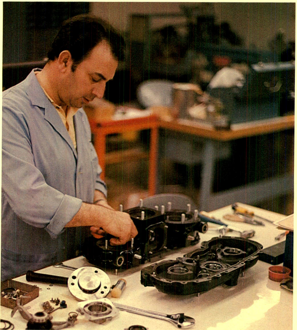
The repair and overhaul of aircraft accessory gearboxes is an important part of Spar's activities.
