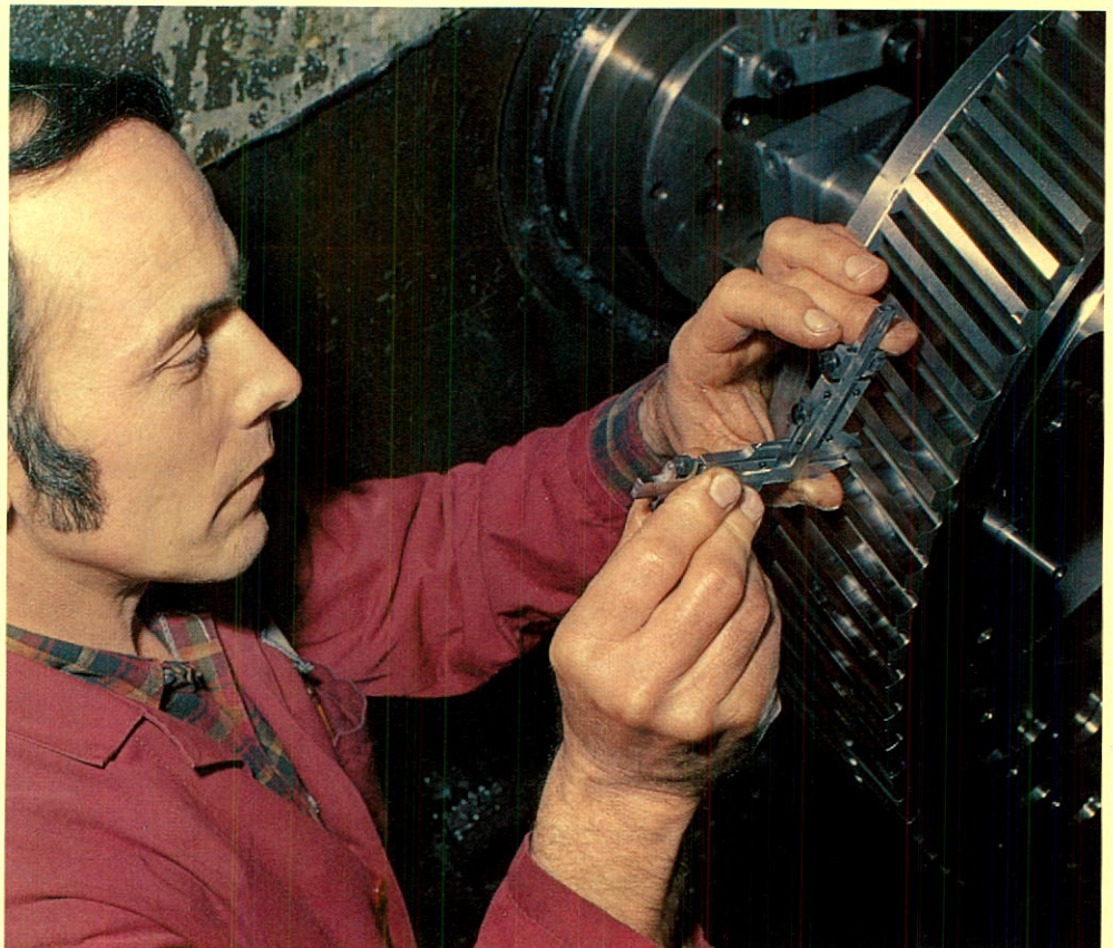
Checking a conformal gear for a Westland Lynx helicopter at Spar's Manufacturing Division.
