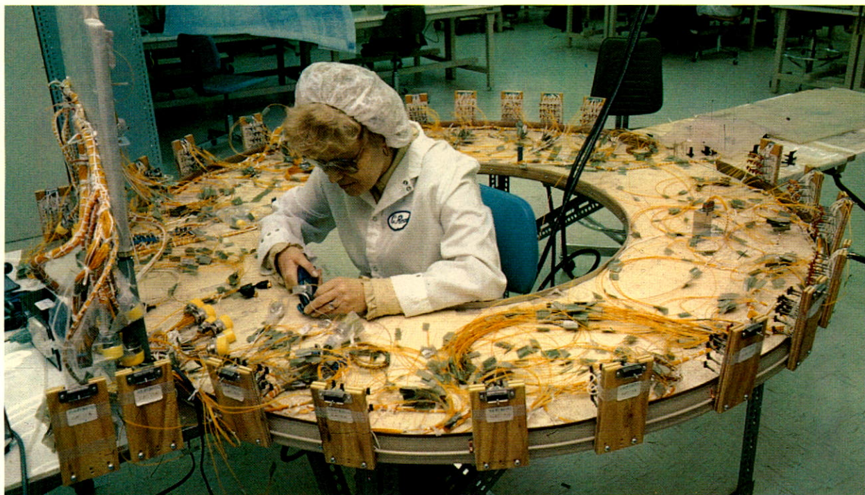
Anik D wiring harness for de-spun shelf at Spar's Kanata plant.
