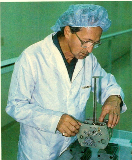
Final assembly of a STEM mechanism for the University of Tokyo's EXOS-C spacecraft in Astro's clean room, Carpinteria, California.
