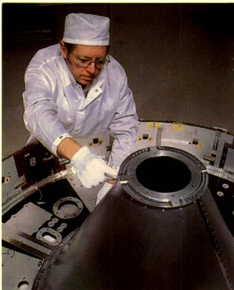
Spar technician working on upper cone on de-spun shelf on Anik C satellite structure.
