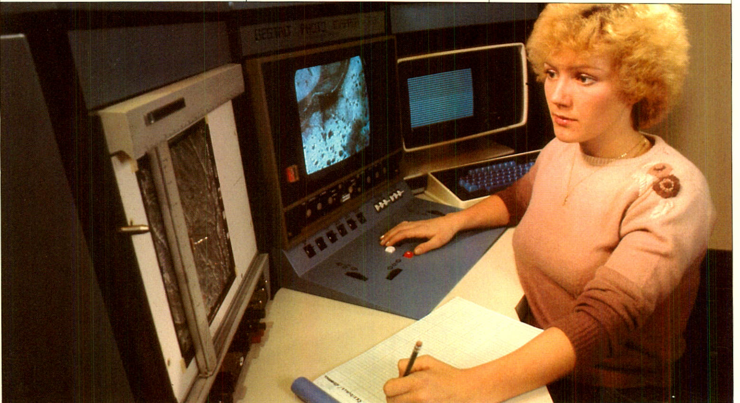
The Series IV Gestalt Photo Mapper (GPM), at Northway-Gestalt's Toronto operation, is a unique electronic system that scans aerial photographs, removes inherent distortions, reshapes the image and produces an orthophoto — a map-accurate image of the terrain.
