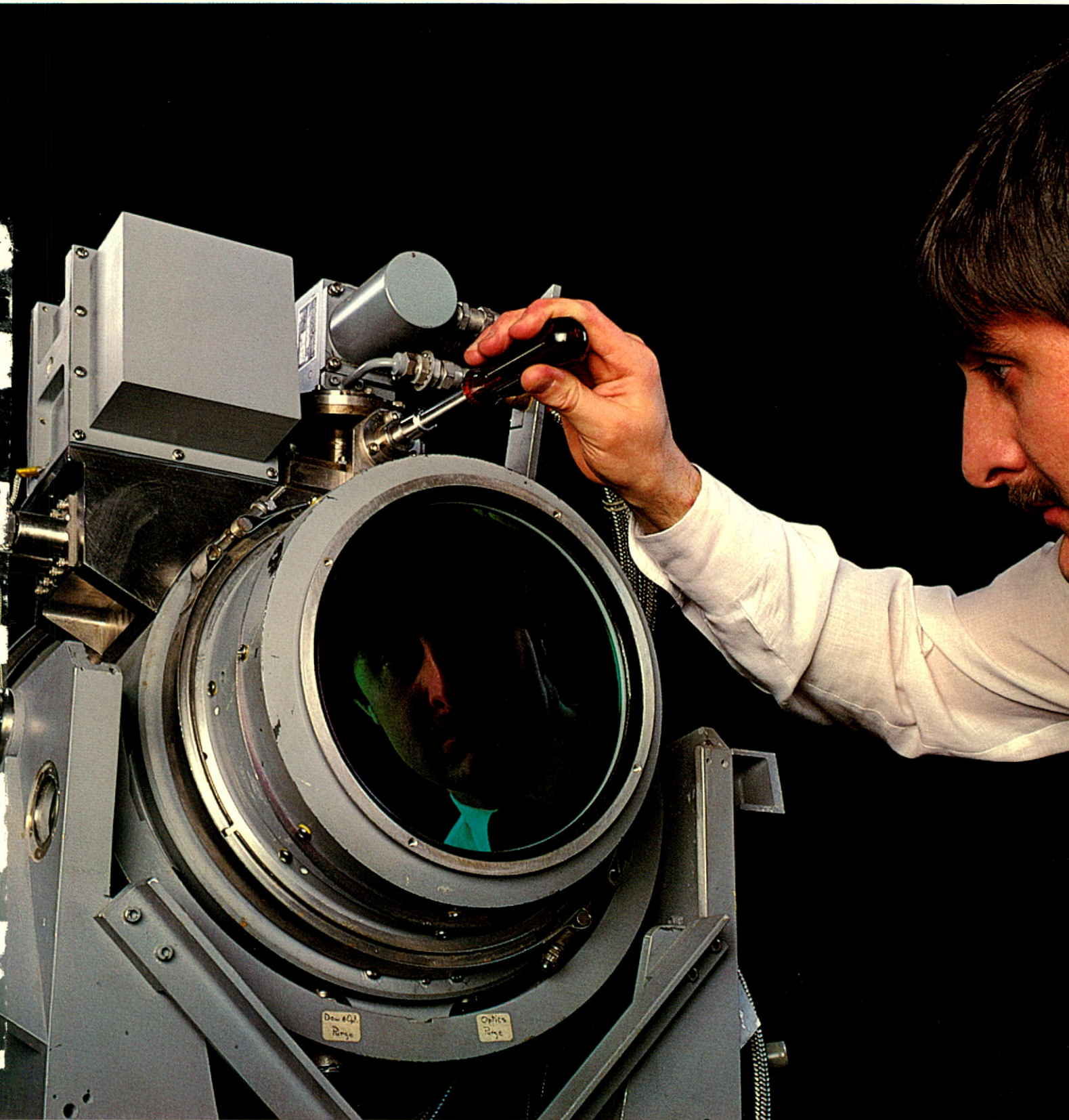
Spar has developed a unique infrared surveillance system for the passive detection of ships, missiles and aircraft for defence and navigation purposes.
