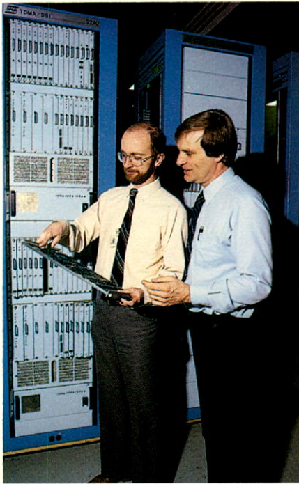
Peter Garland and John Barkwith examine a printed circuit board of Spar's Time Division Multiple Access equipment.
