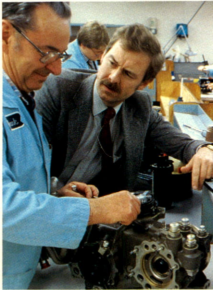
CF 18 generator overhaul
