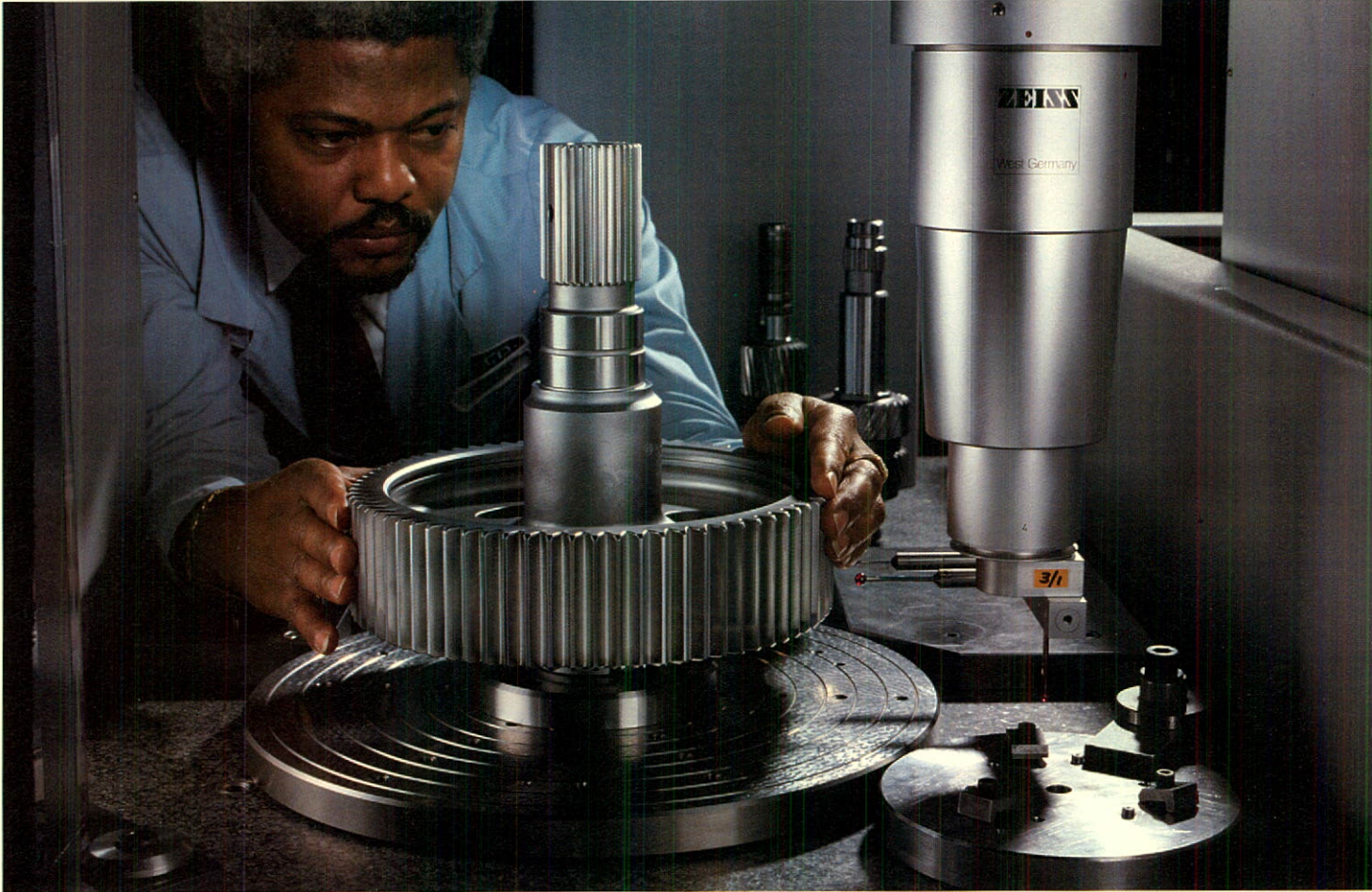
Melvin Waldin sets up to check dimensions of a Boeing Helicopter's SR&M gear on the new Zeiss universal coordinate measuring machine.
