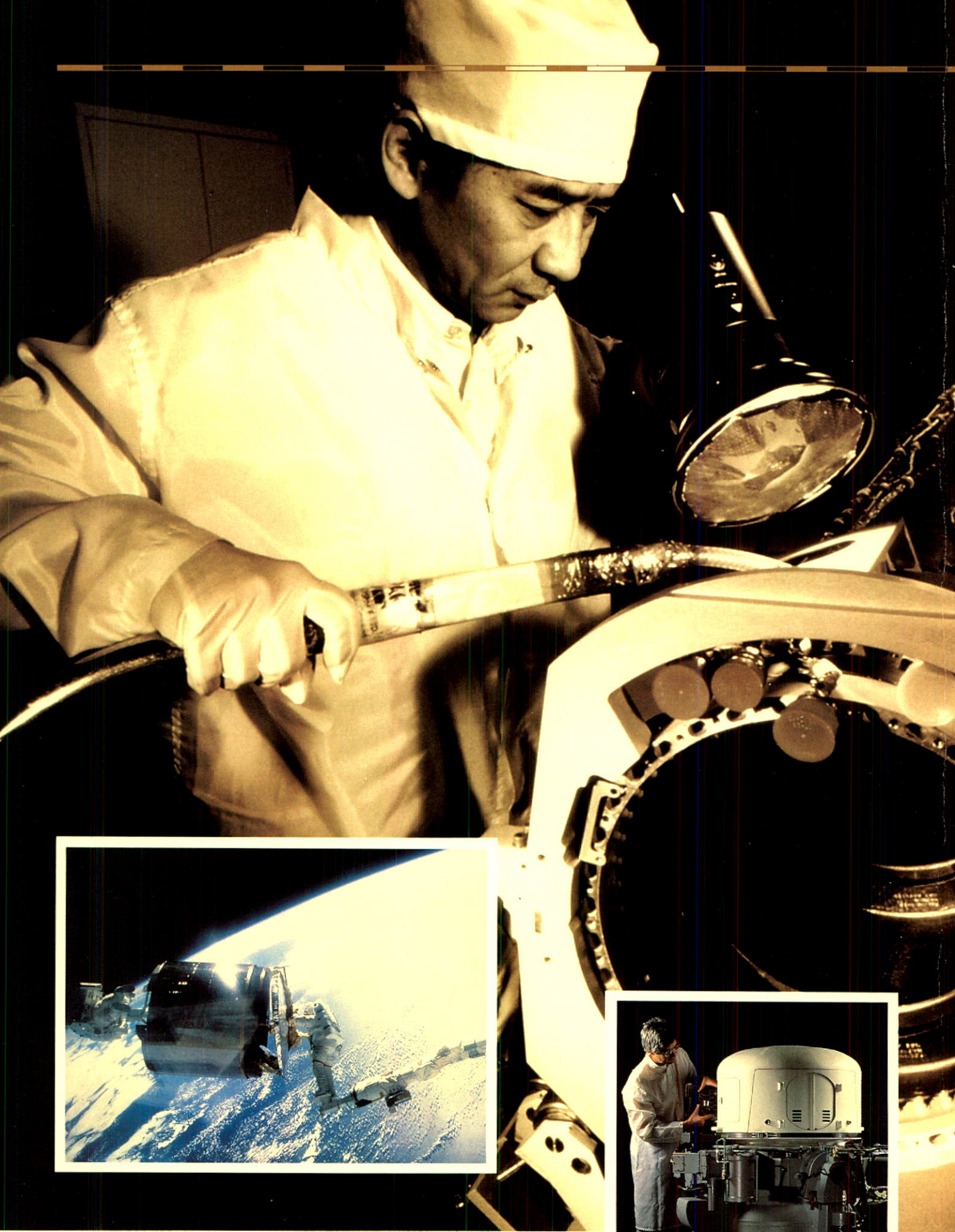
Large photo: Shuttle Remote Manipulator System (SRMS) undergoing cleaning and black light inspection by ATSG technician Chen Huang.
