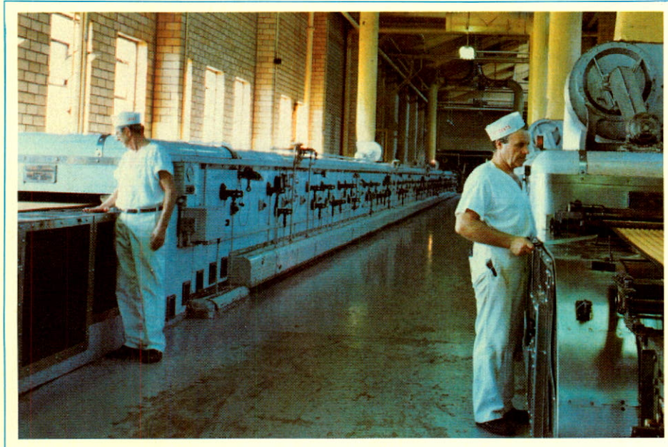
In the Christie Brown & Co. Ltd. Etobicoke plant, steady streams of biscuits are baked in precision-controlled ovens fired by natural gas. Quality control, providing uniform texture and appearance, is possible with natural gas in this continuous high-volume operation.
