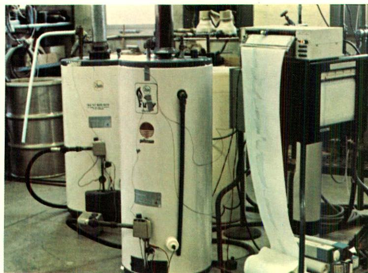
With the cooperation of other utilities, these improved gas fired water heaters are being subjected to tests by the Canadian Gas Research Institute in their laboratory, as well as under field conditions at 34 locations across Canada. The test data is currently undergoing evaluation.
