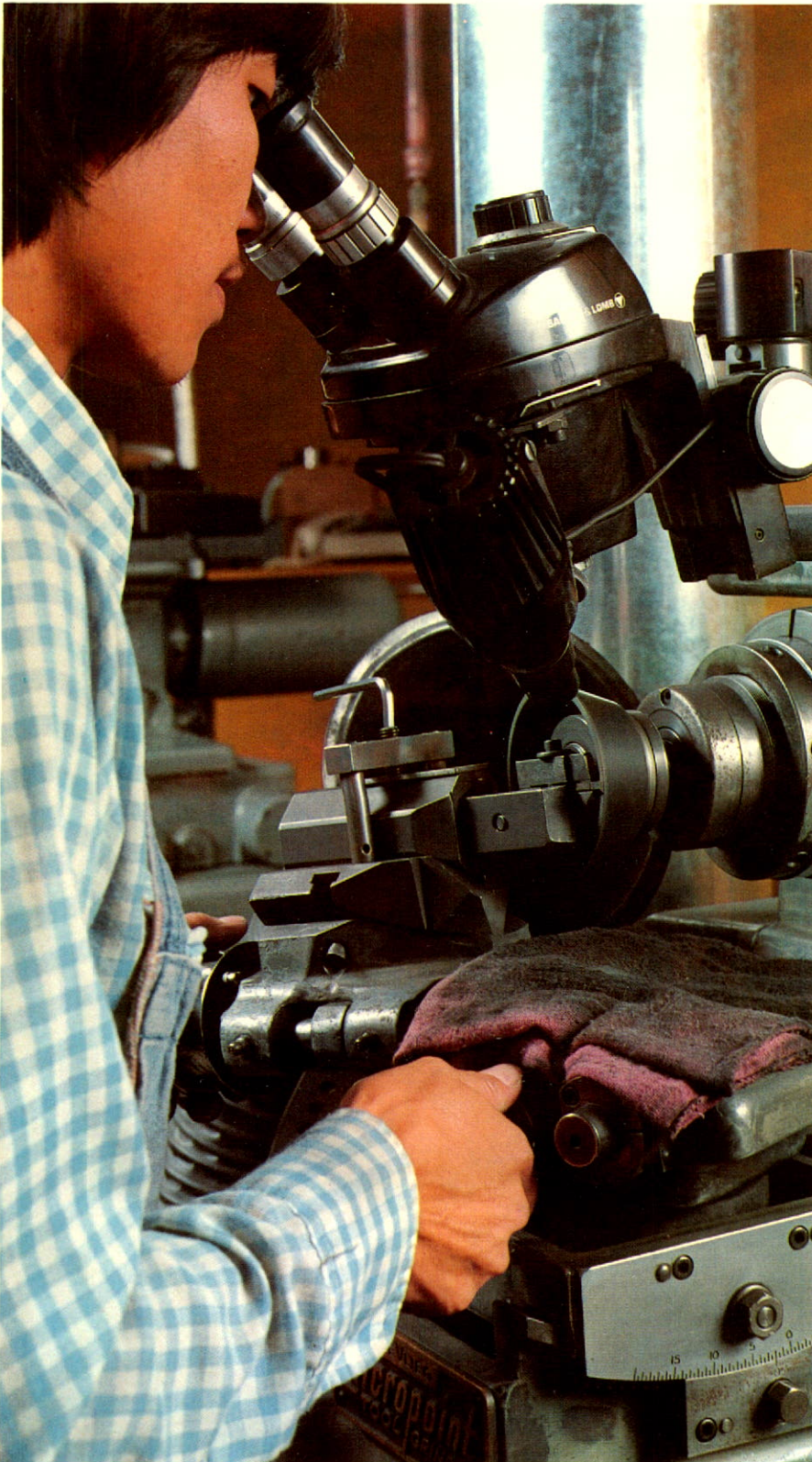
Grinding corner radii on API threading inserts, at Triangle Grinding, Inc.
