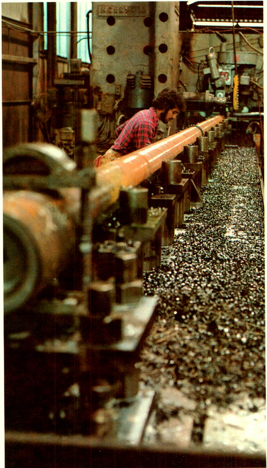
A 5½-inch hex kelly before machining the hex, at OMSCO Industries, Inc.
