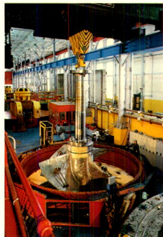
30 ton stainless steel runner for an hydraulic turbine is rated at 13,500 HP under a net head of 26 feet... 12.5% greater than previous designs. Made by GE Canada it is destined for Hydro Quebec's Rivière Des Prairies power plant near Montreal.
