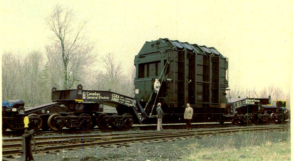
The first of ten 735KV generator transformers for Hydro-Québec's LG3 James Bay Generating Station being shipped on the Power Transformer Section's new depressed centre rail car.
