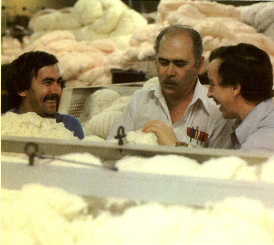
▲Half of the Sorel plant's employees are engaged in a series of operations which are collectively referred to as spinning. Here employees in the opening and blending operation process staple fibres which will eventually be spun into yarn.
