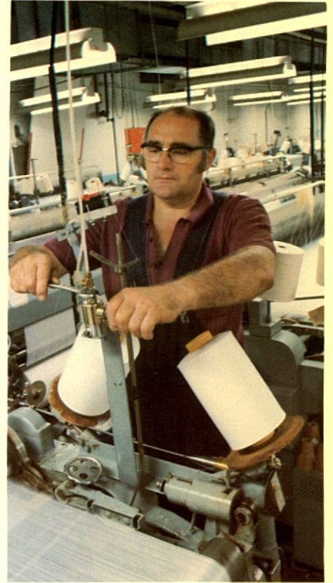
▲High-speed, shuttleless, water jet looms at our Coaticook weaving plant produce polyester and acetate fabrics.
