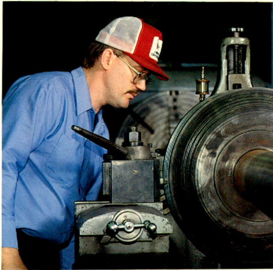
Lathe operator Greg Jordan prepares a power piston for a compressor engine.
