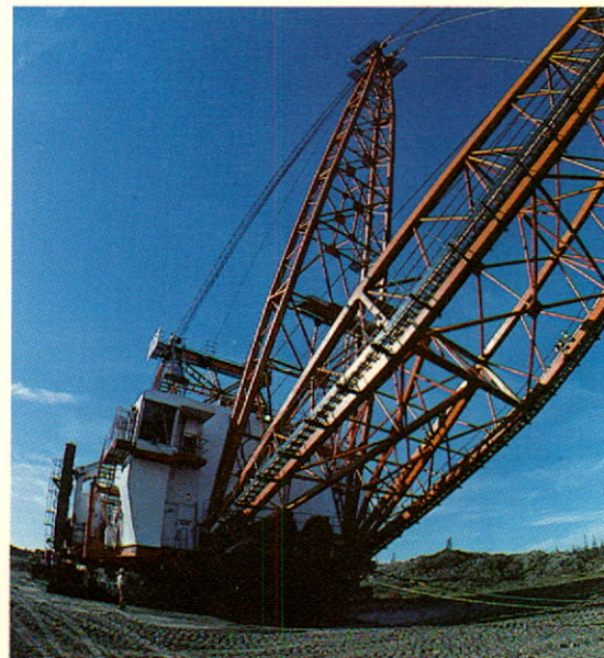
Pine Point, N.W.T.: the 30-cubic-yard dragline \Delta removes overburden at the largest mine in the Territories.
