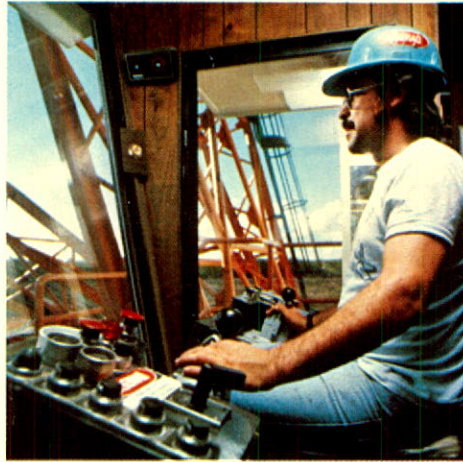
Operator maneuvers 30-cubic-yard dragline at Pine Point, N.W.T. where a record seven million tons of waste and overburden was removed in 1980.
