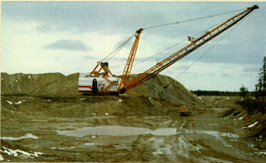
The new 30 cubic yard "walking" dragline at the Pine Point zinc-lead mine dwarfs every machine on the property, including this large tractor.
