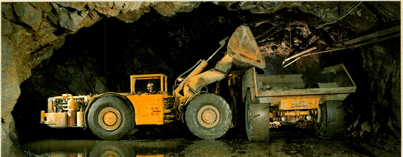
A modern scoop tram loading ore in the Sullivan mine at Kimberley, B.C.
