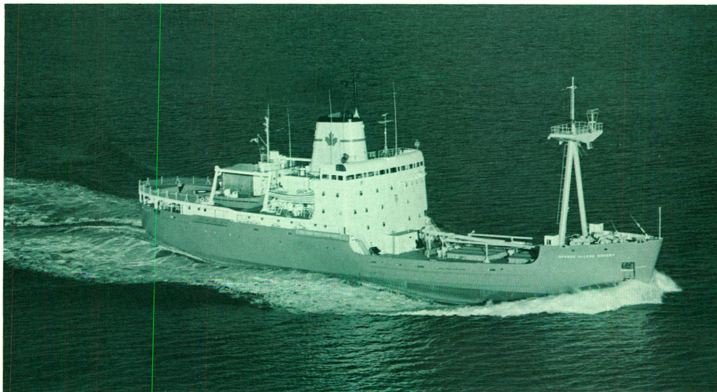
Canadian built "Norman McLeod Rogers" is the first icebreaker in the world to be driven by gas turbines. Manufactured in Hamilton, these turbines provide extra muscle for crashing through heavy ice.
