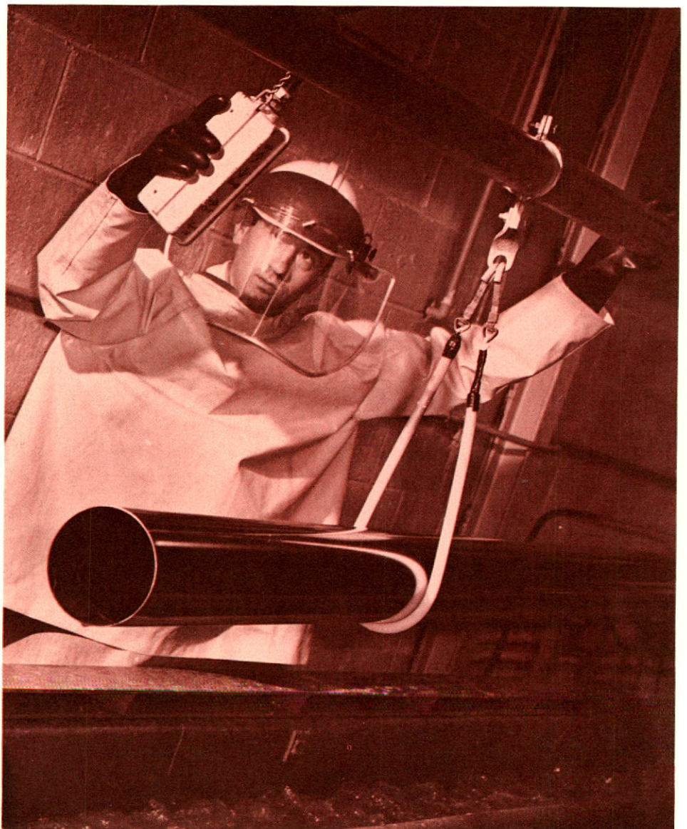
Exotic metals and special techniques are used in making atomic reactor components such as the calandria tube, above. These tubes hold the nuclear fuel bundles which power the reactor.
