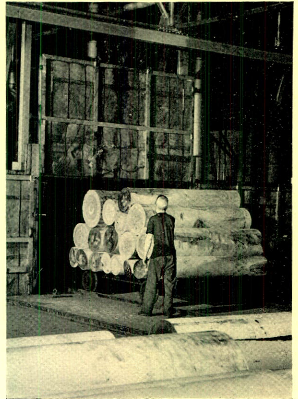
Logs Being Placed in Vat for Steaming
