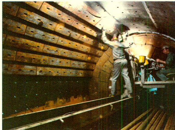
(Below left) Ni-Hard mill liners cast by Foundry are used in rod and ball mills to grind ore to a fine powder.
