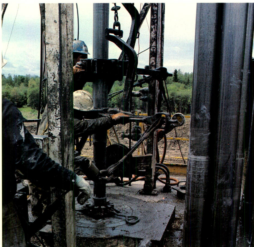
Drilling crew making drill pipe connection on rig at Drayton Valley, Alberta.
