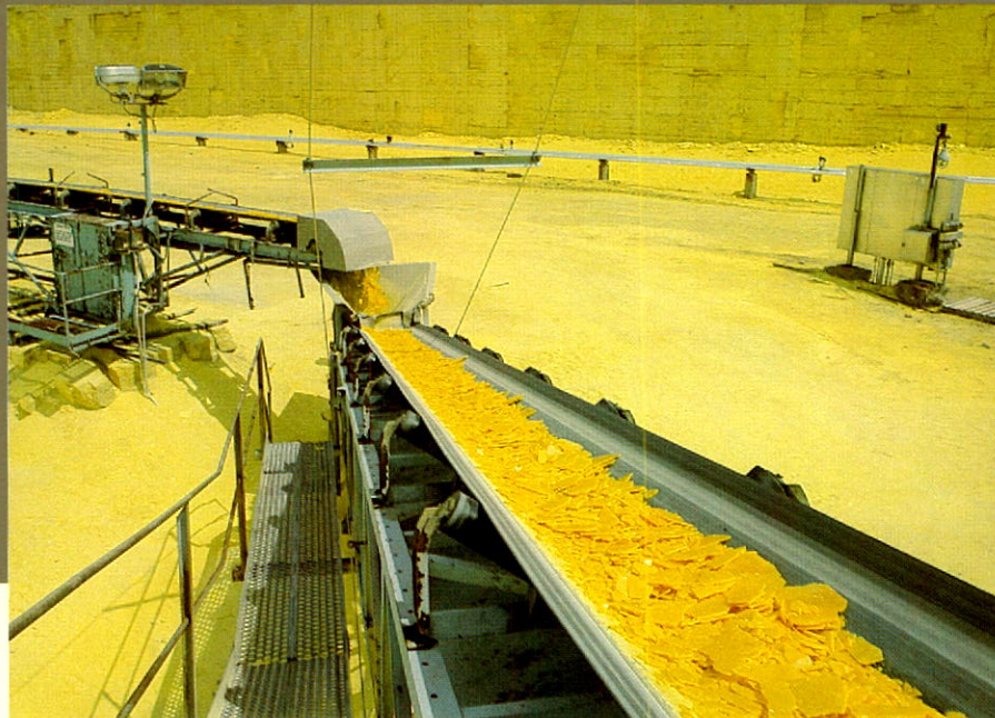
Moving slated sulphur to stockpile at Petrogas plant, near Calgary.
