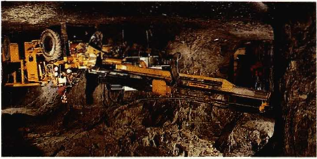
Jumbo drill with three 20-foot booms in Sullivan Mine.
