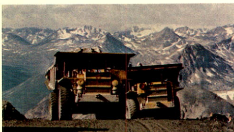
The plunge of the orebody into the side of McDame mountain requires the removal of massive quantities of waste rock to sustain continuous ore mining. This mine truck hauls an 85 ton load to the waste dump, part of over 500 such loads every day throughout the year.
