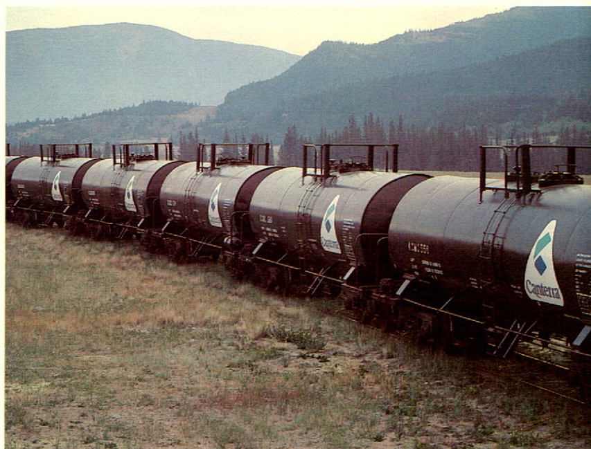
Liquid sulphur is shipped to domestic markets in tank cars like these ones which have been newly painted with the Canterra logo.
