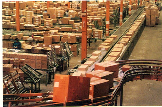
New computer-controlled conveyor system in the Bay's Toronto distribution centre.
