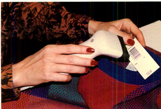
Hand-held wands at point-of-sale read bar code information and speed customer service.
