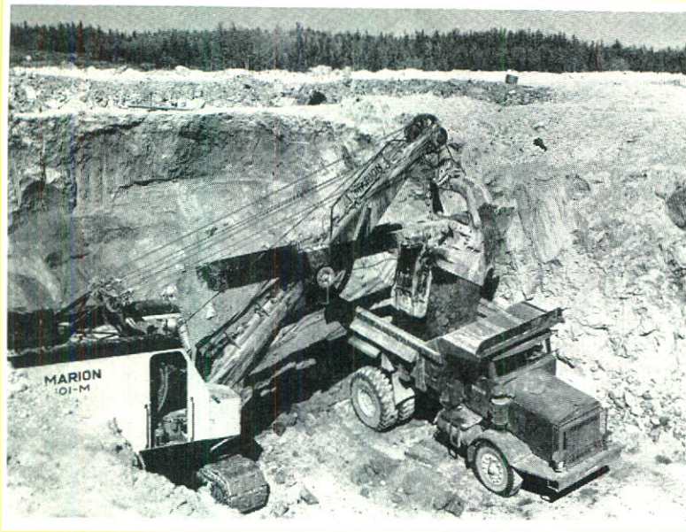
A power shovel loads a Euclid ore truck, which will carry 25 tons.
