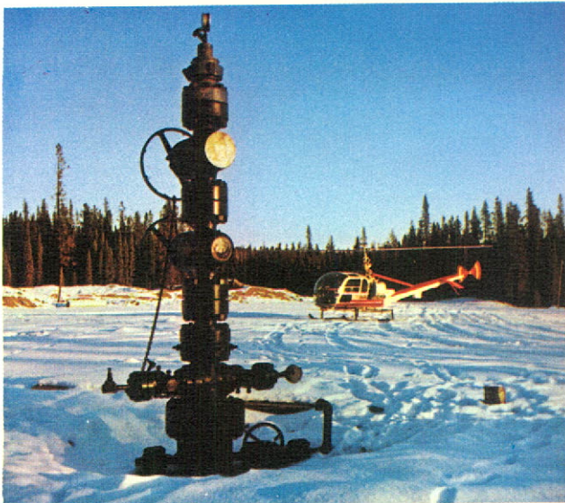
The wellhead at Gulf et al Strachan 11-22. UBR holds a 33.75% working interest in this well which encountered over 600 feet of gas pay zone in the Leduc Reef.
