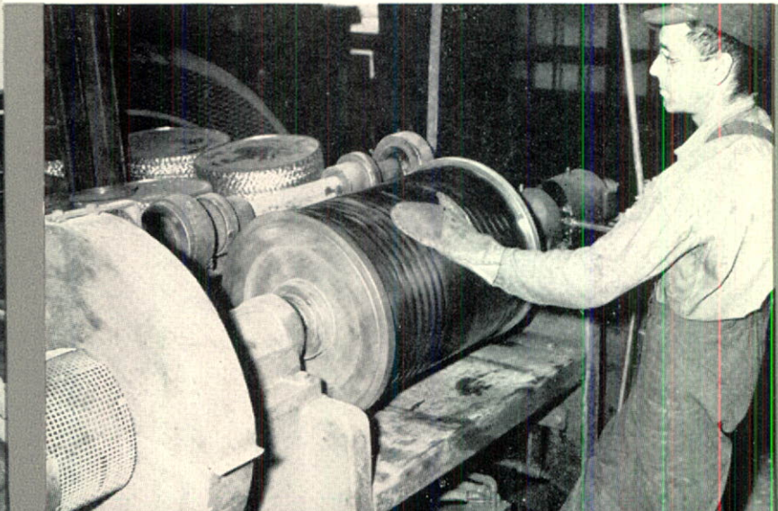
Making steel drums for shipment of Shawinigan carbide.
