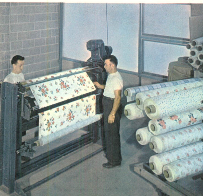
Inspecting printed and embossed 'Vinylite' film at the converting plant of Canadian Resins and Chemicals Limited at Ste-Thérèse.
