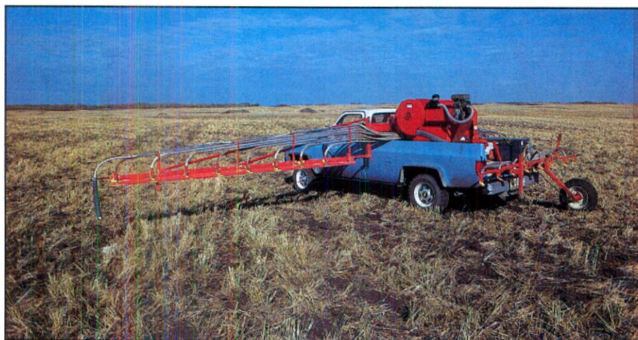
Valmar Spreader mounted on a pickup is available from some UGG elevator managers for fast, easy application of granular herbicides.
