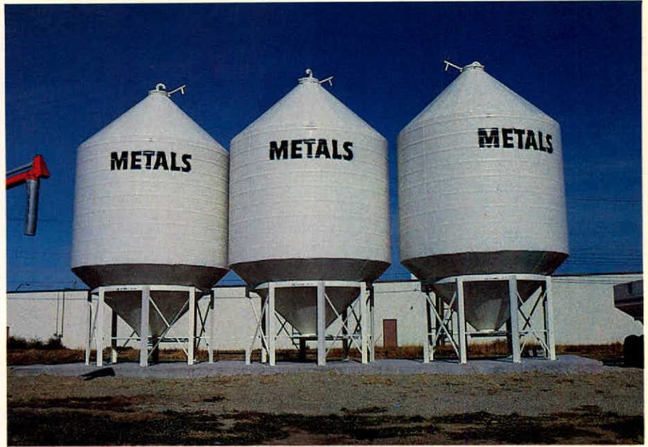
Fertilizer hopper bottomed bins, like these at Morden, Man., were installed at 24 points this past year.
