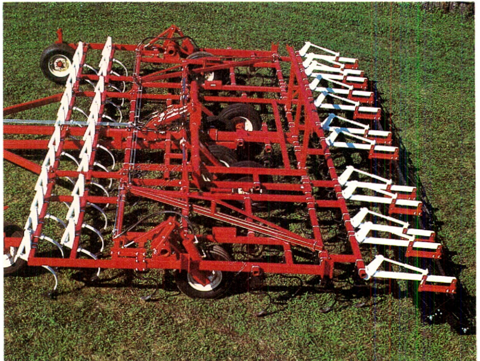
Soil conditioners are becoming popular for incorporating herbicides. It's a combination of a field cultivator in front, followed by a ground driven spiral reel and spike tooth harrow at the rear.
