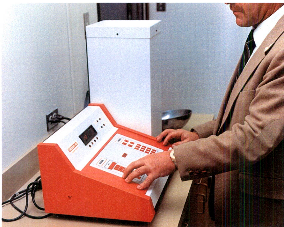
A new type of grain protein analyzer is being tested for use at country elevators. An unground sample of wheat poured into the hopper gives a protein content readout in about 30 seconds.
