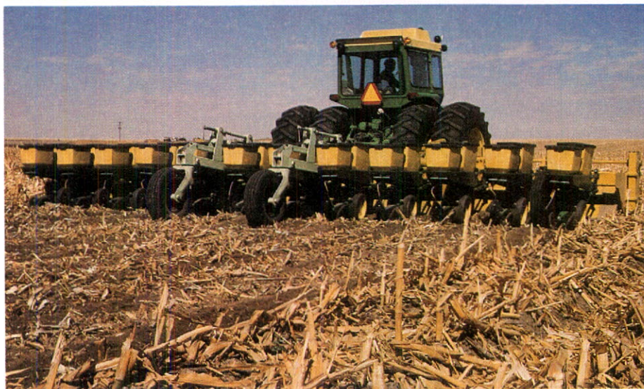
Farm machinery continues to get bigger and more complex. Top left: A 60-foot tractor mounted swather; top: This 100-foot wide cultivator is pulled by a big Steiger tractor; and left: a minimum tillage system works stubble, prepares a seedbed, applies and incorporates herbicides and plants up to 12 rows all in one operation.
