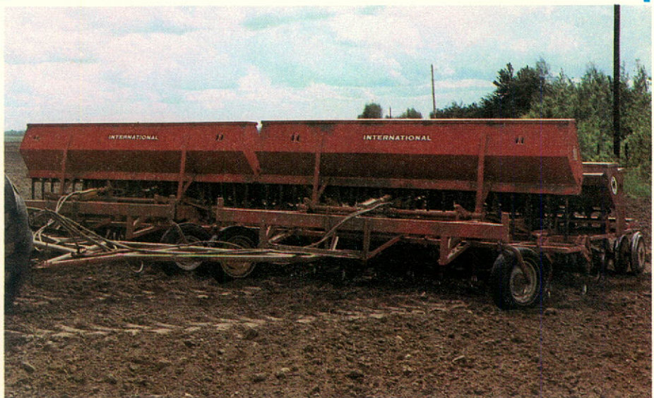
Fertilizer applicators are now available to band fertilizers just to the side and below the seed during seeding with a disc press drill.
